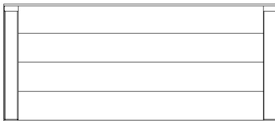
RP3 | PANEL DE TECHO - W2A03267 (2) | 1 5/8"x20 5/8"x59" (42x524x1204)
